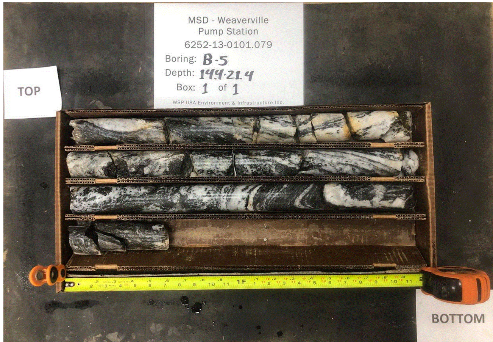
Rock core from 14.4 to 21.4 feet (going left to right and top to bottom) boring B-5.
