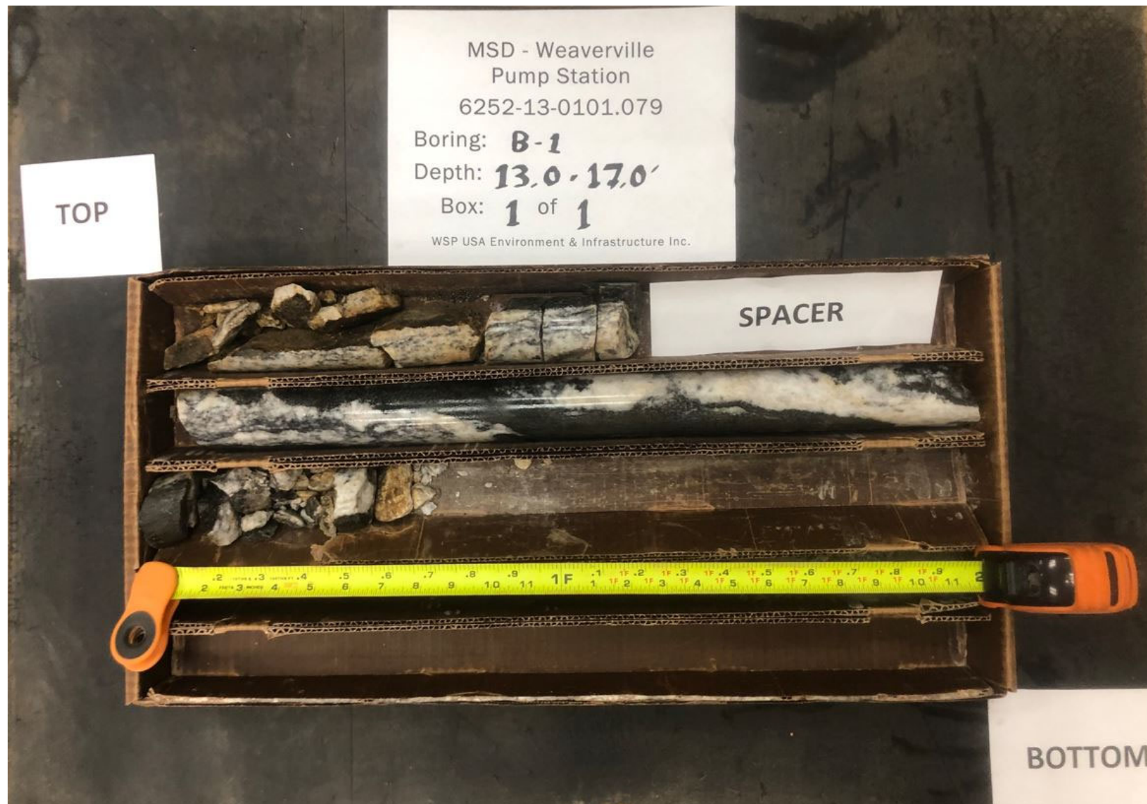
Rock core from 13.0 to 17.0 feet (going left to right and top to bottom) boring B-1
