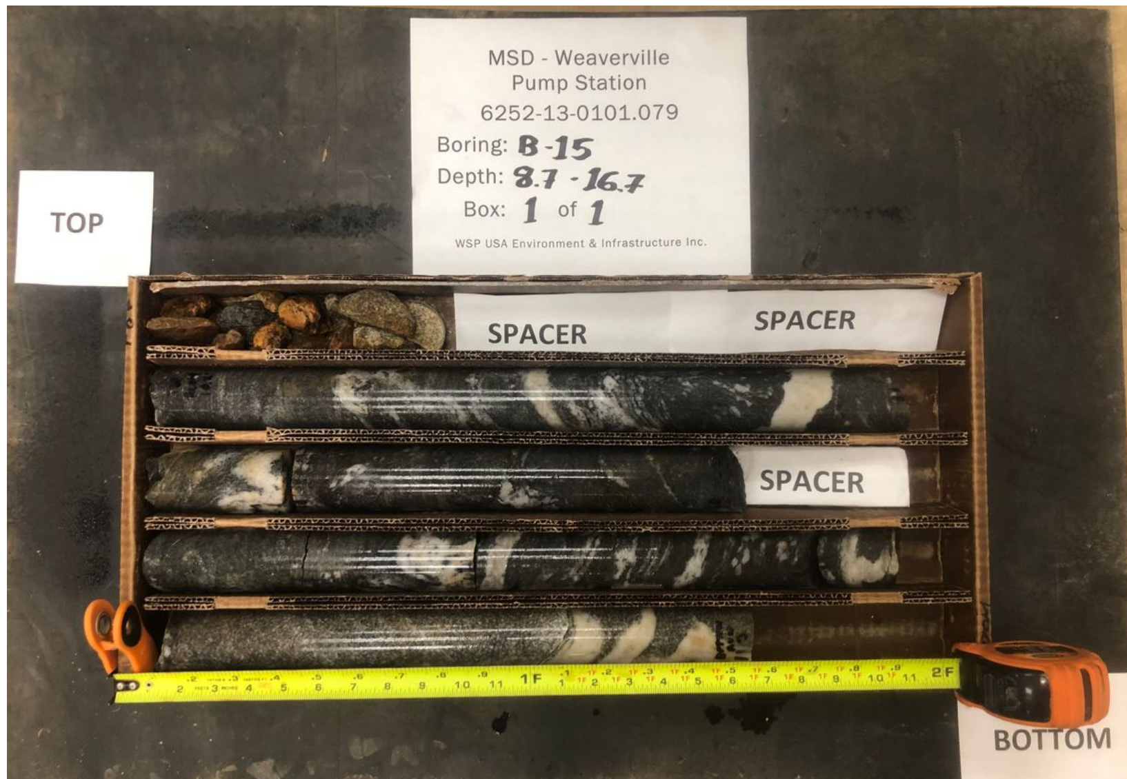
Rock core from 8.7 to 16.7 feet (going left to right and top to bottom) boring B-15.
