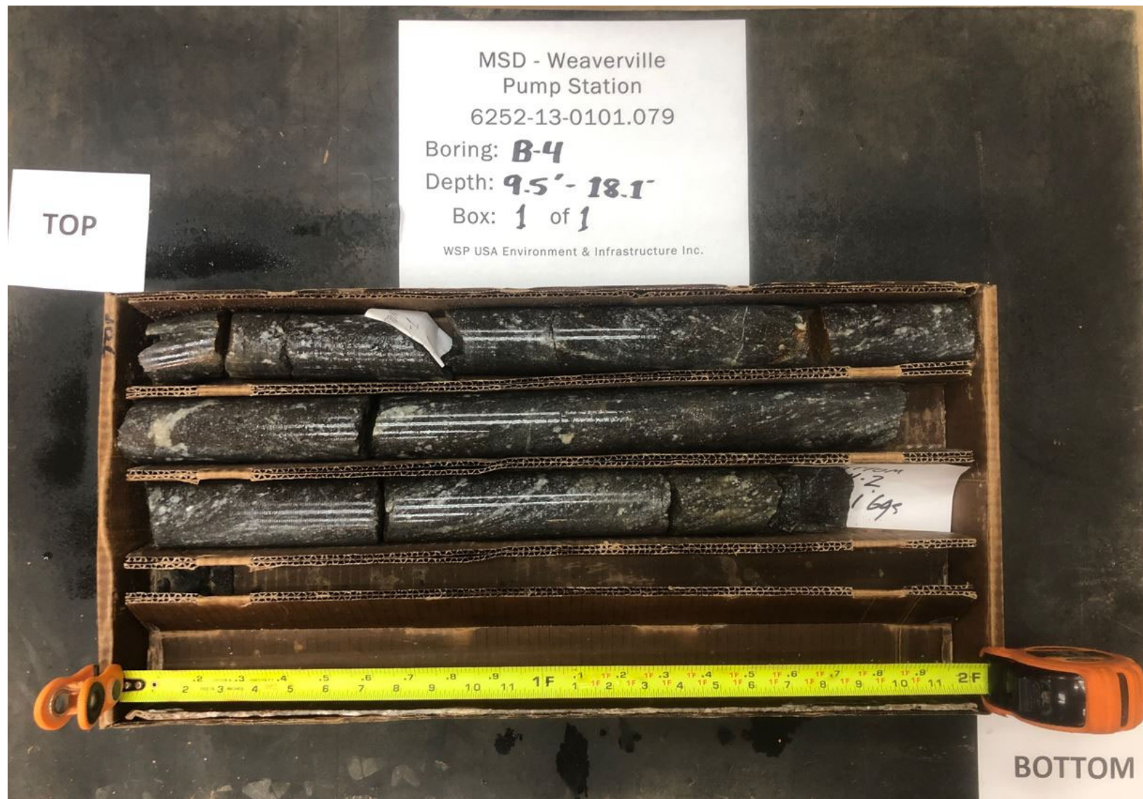
Rock core from 9.5 to 18.1 feet (going left to right and top to bottom) boring B-4.
