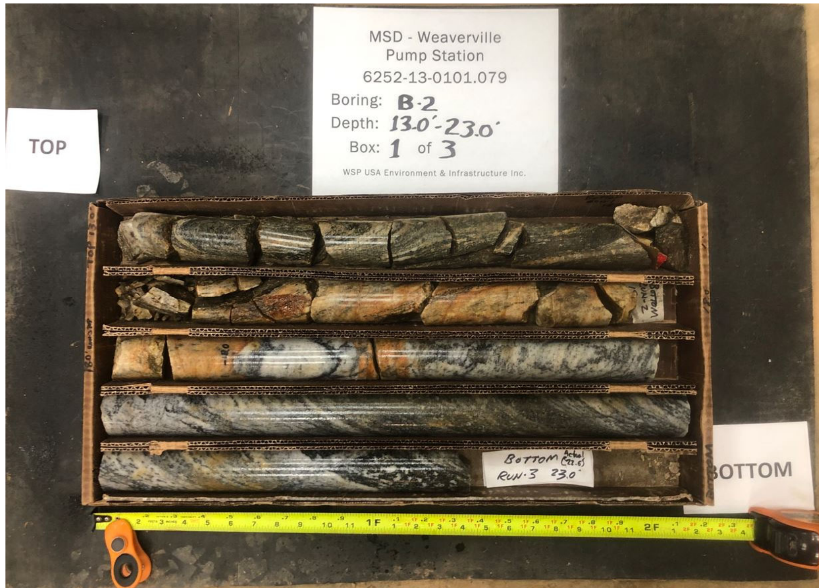
Rock core from 13.0 to 23.0 feet (going left to right and top to bottom) boring B-2.
