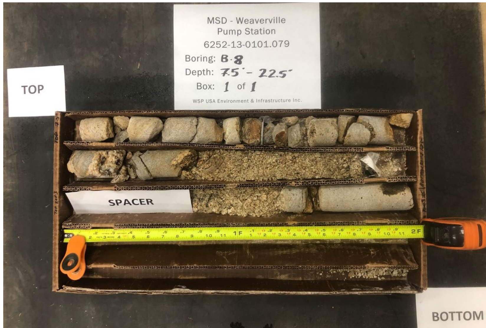
Rock core from 7.5 to 22.5 feet (going left to right and top to bottom) boring B-8.
