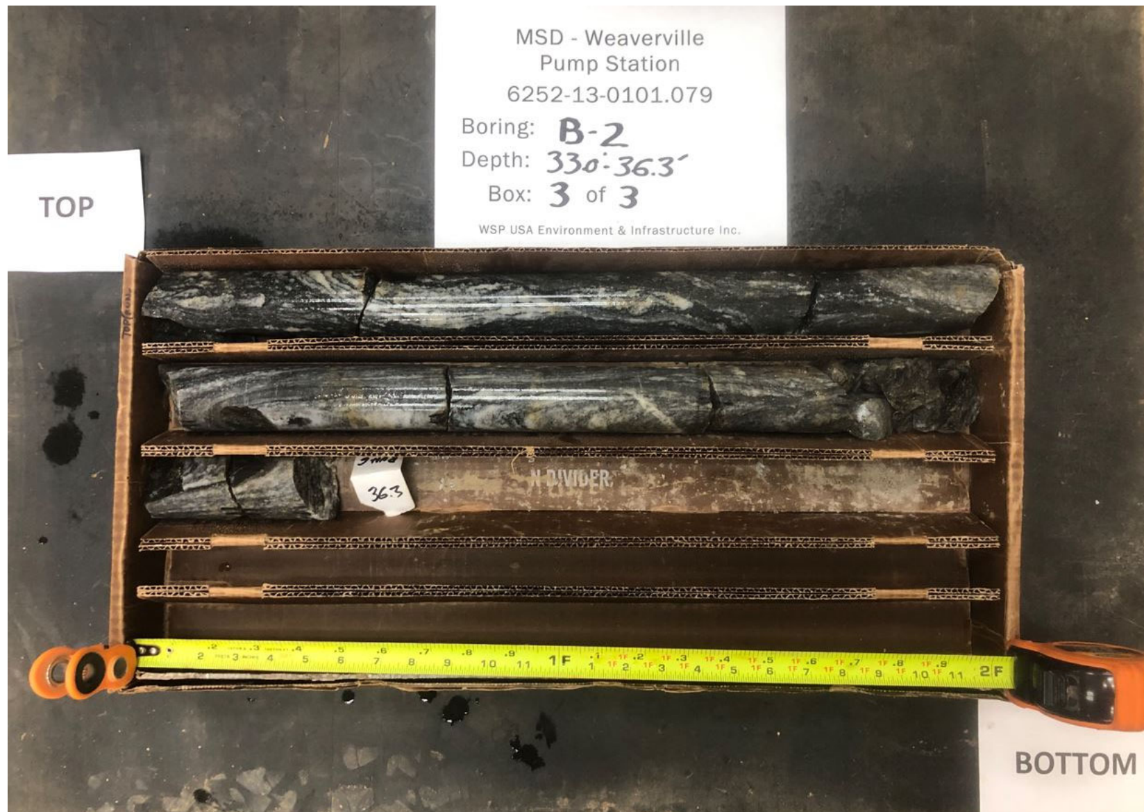
Rock core from 33.0 to 36.3 feet (going left to right and top to bottom) boring B-2.
