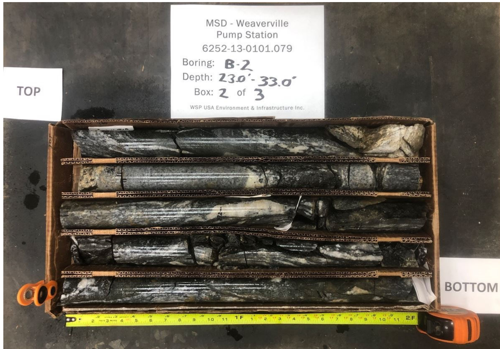
Rock core from 23.0 to 33.0 feet (going left to right and top to bottom) boring B-2.
