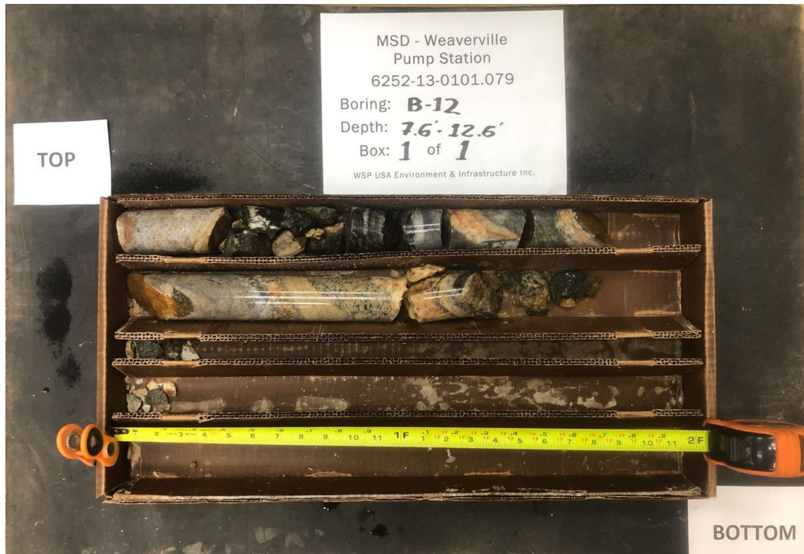
Rock core from 7.6 to 12.6 feet (going left to right and top to bottom) boring B-12.
